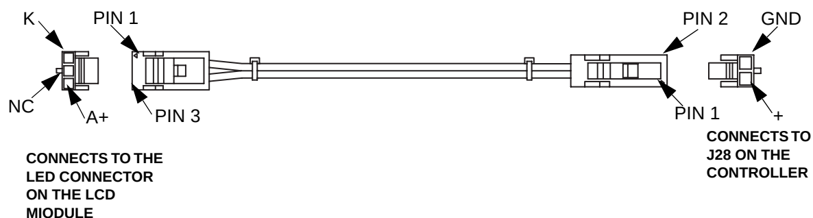
Figure 8-58: LCD Backlight Cable Wiring Diagram
