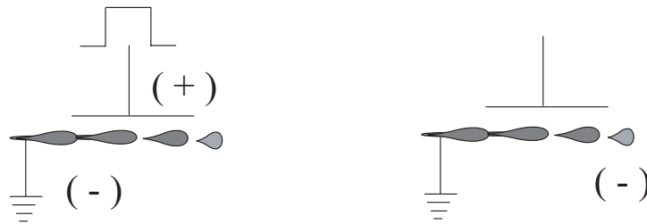
Figure 4-2: Charge Tunnel Operation
